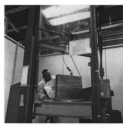
"OLD SAND POUNDER" is the oldest drop testing machine at Sandia Laboratory. Here E. W. Upchurch readies the machine for a test. The machine will give a 150-lb. test unit a velocity change of 30 ft. per second. It has been used at Sandia for over 10 years.
